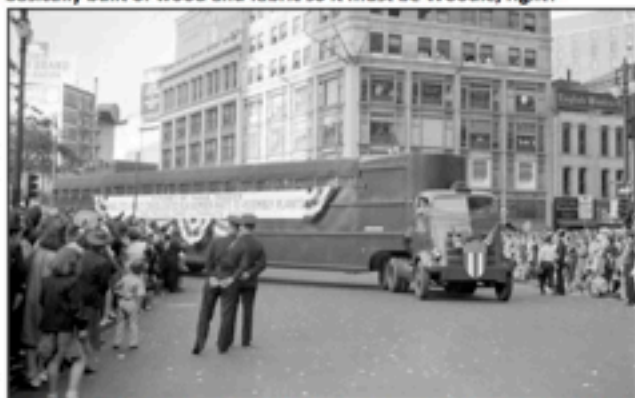
A specially designed and built dual engine Ford COE was used to haul Ford-built B-24 bomber subassemblies built at Willow Run to assembly plants in Texas and Oklahoma.
